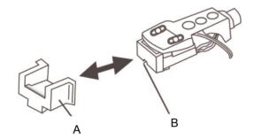
Š It is recommended that you put the stylus cap back on after playing a record to protect the stylus **B**.
